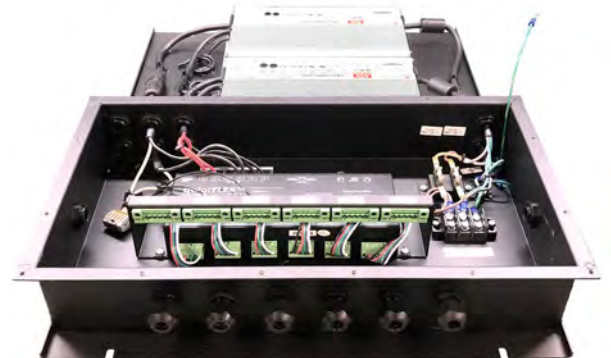
Custom low voltage QolorFLEX Dimmer boxes
